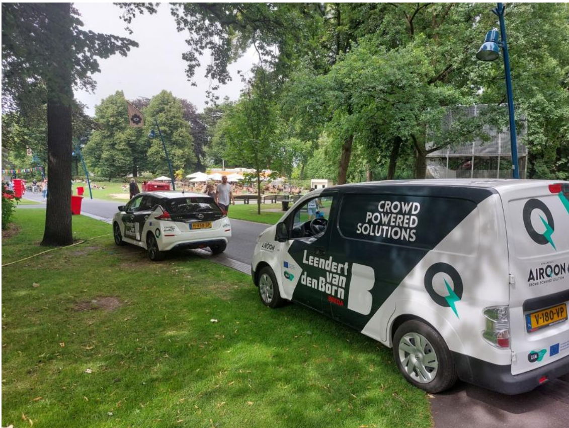
AirQon can deliver power to events by means of cars, providing energy directly, and vans, acting as energy buffers (Source: facebook.com/airqon)
