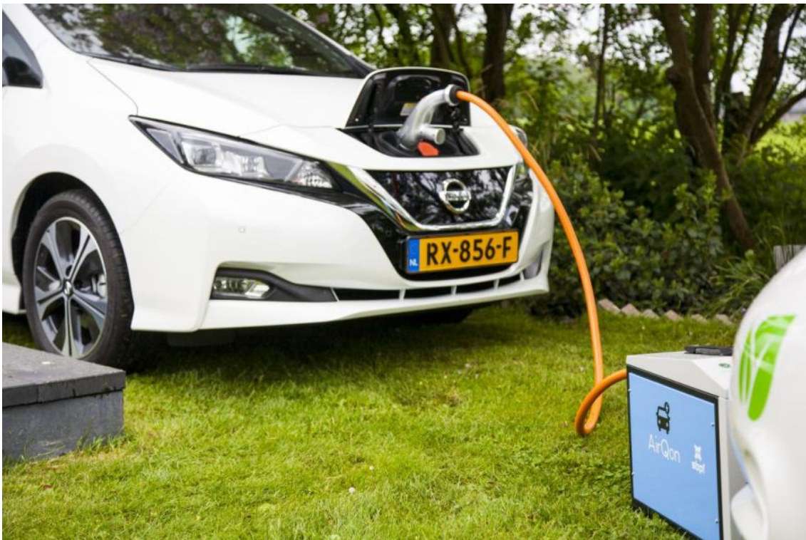
One of the first prototypes of AirQon device delivering power from a car (Source: facebook.com/airqon)
